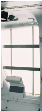
Equipment rail (Wdw): 10.0kg payload / ea
